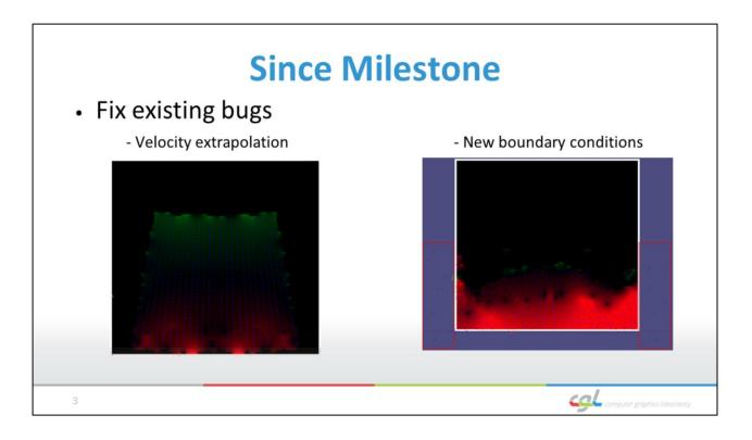
Since then, we first fix the existing bugs by extrapolating the velocity field in the air-fluid surface as suggested by vinicius. Indeed it really helps. We also set more advanced boundary conditions so that particles won't go out of the box.
