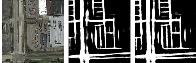
Figure 4. Left: original image. Middle: results using only CRF in [2]. Right: result of our approach. (Parameters of post-processing modules in the middle and the right are both tuned on local validation set)
